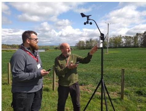
Using the agri-tech weather station set up in the fields, the weather stations provide reliable, accurate, ultra-local data remotely. This data gives farmers their decision-making power back. It streamlines their daily tasks, rationalises the management of chemical inputs, helps them care for their crops and boosts their productivity.
